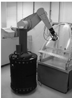
Figure 1. A mobile manipulator consisting of a PUMA 560 mounted on a Nomad XR4000 polishing an aircraft canopy with a curved surface geometry that is unknown to the mobile manipulator. The polishing tool attached to the arm end-effector moves in a compliant scrubbing motion while maintaining a desired normal force on the aircraft canopy. The mobile base is guided by the human operator to polish the to desired areas on the canopy surface.
