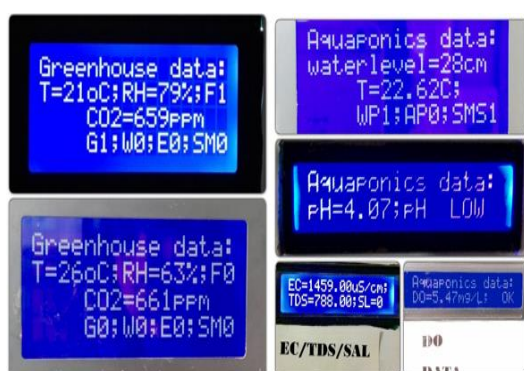
Fig. 4. Sample Aquaponics Greenhouse data and status of actuators taken on a typical winter day as displayed on an LCD
