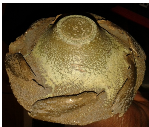
Fig. 6 A worn out impeller
