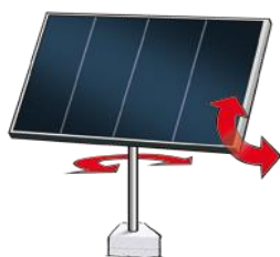
Figure 1: a dual axis solar taking mechanism. Source [10]
