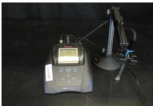
Figure 2: Thermo scientific Orion star pH meter
