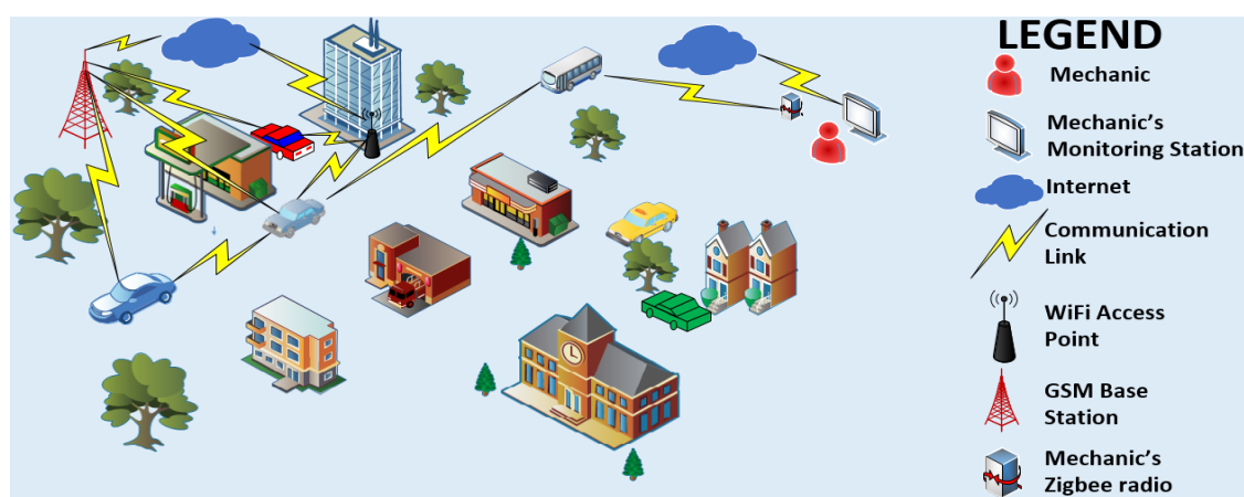
Fig. 1: A real community showing the vehicle monitoring system using GPRS, Wi-Fi and Bluetooth and Zigbee relay systems
